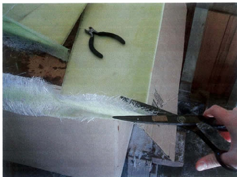
Applying final patches of fibber glass to the ends and leading edge
