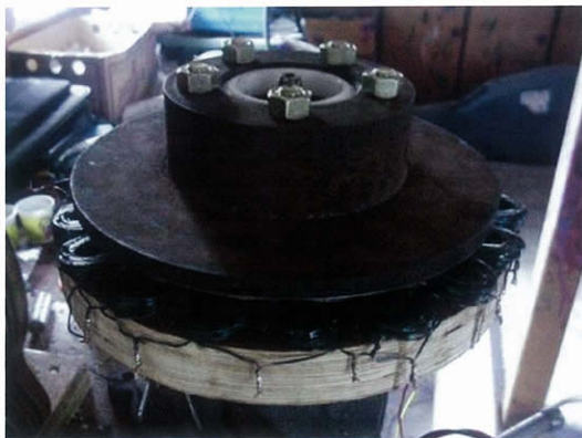
Homemade Volvo Brake Disc PM alternator, 800 watts, $150!
