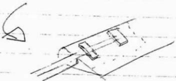
With a patch of fibreglass underneath the steel and then another coat of fibreglass over the entire blade, which should give a very strong set up.
